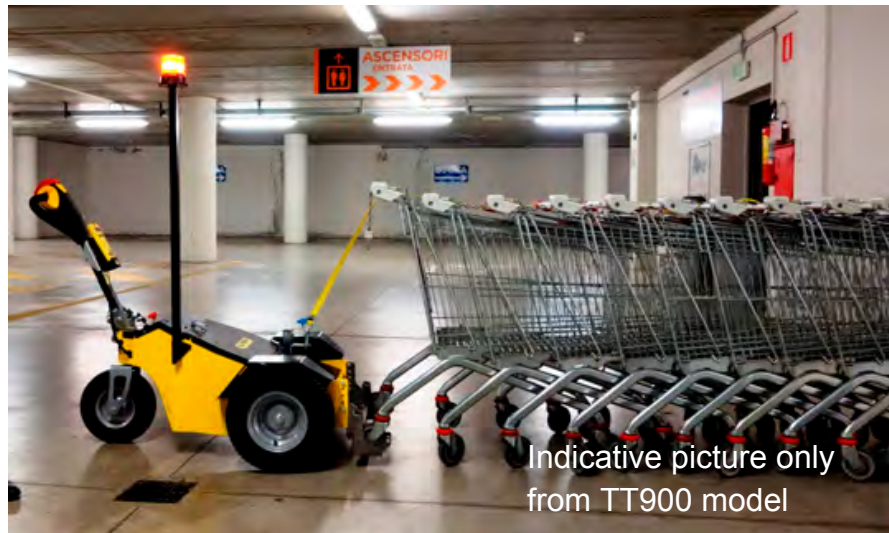
Optional Remote Control & Flashing Light on Pole For Alitrak Tow Tugs
