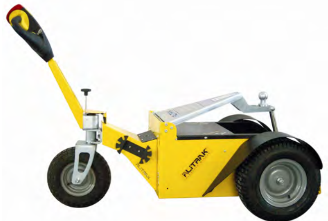
Pivoting wheel allows a minimum of space to steer
