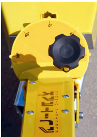
Horizontal adjustment of the tiller, to facilitate the towing of bulky loads.
